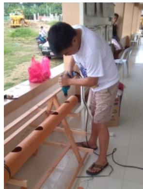
Figure 3. Hydroponic Structure with Polyvinyl Chloride
